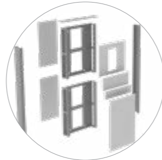
Removable/lockable panels for maintenance
